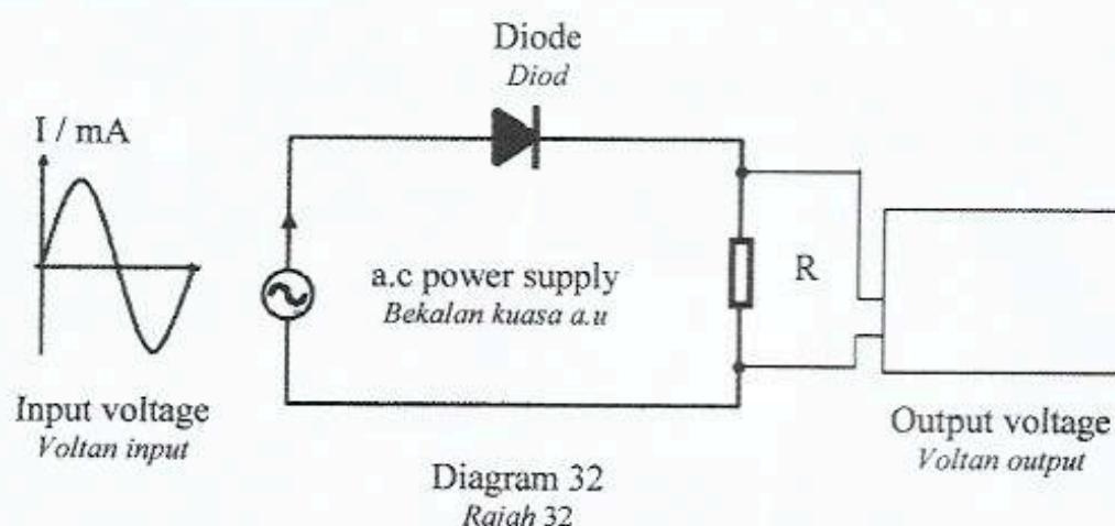
Which graph shows the correct output voltage?
