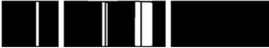
Spektrum cahaya lampu merkuri Spectrum of mercury lamp
