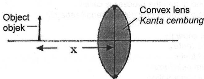
The image formed is **virtual** and **enlarged**. The object is at
