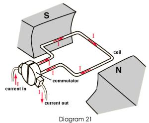
Using the concept of the magnetic effect of an electric current, explain with the aid of diagrams how forces are produced on a wire in the coil, as shown in the diagram above.
