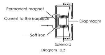
Explain the working principle of the telephone earpiece.
