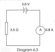
Calculate the internal resistance of the battery in the circuit above.
