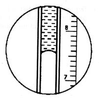
Diagram 1.5 Air column length reading at 20 °C
