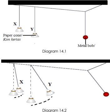
Using Diagram 14.1 and Diagram 14.2, compare the length and frequency of pendulum X and pendulum Y to the length and frequency of the metal bob pendulum. Compare the amplitude of oscillations between pendulum X and the pendulum Y. Deduce the physics concept that involved in the situation.
