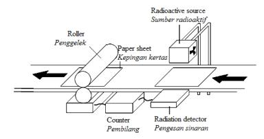
Explain how Strontium-90 is used to measure the thickness piece of paper?
