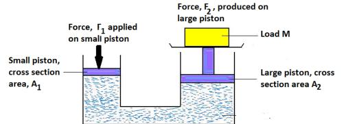
Explain how the hydraulic jack can be used to lift load M when force is applied on the small piston with cross-section area  $A_1$ . In your explanation, state the reason why force  $F_2$  is greater than force  $F_1$ .
