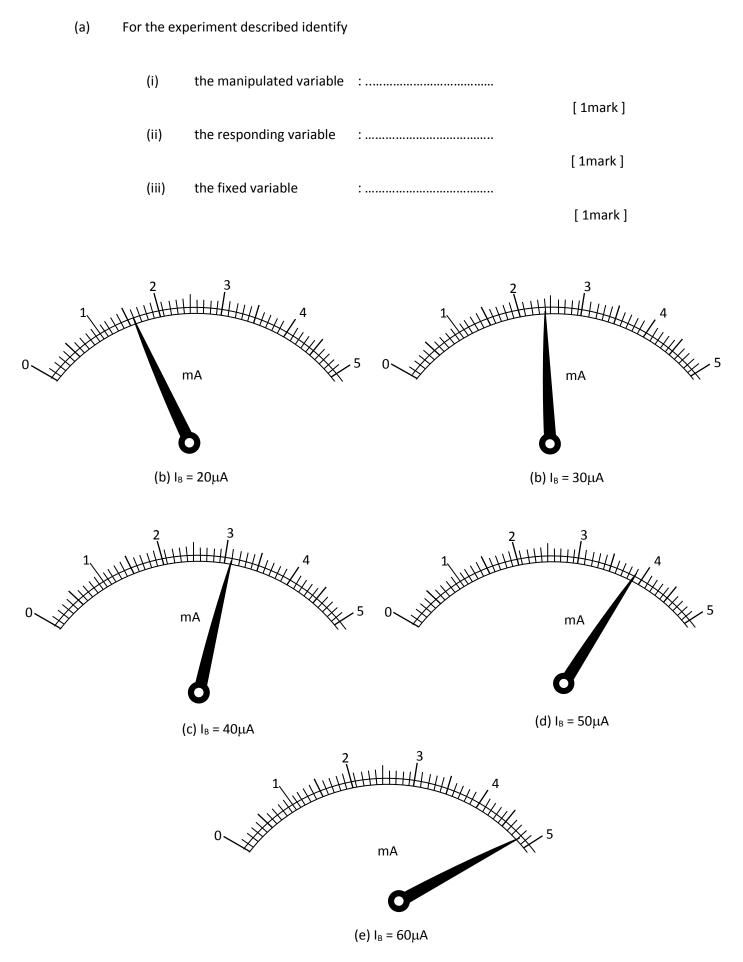
(b) From the diagram, record the collector current,  $I_c$  when  $I_B = 10, 20, 30, 40, 50$  and  $60\mu$ A. Tabulate your results for  $I_B$  and  $I_c$  in the space given below.
