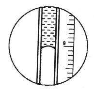
Diagram 1.10 Air column length reading at 70 °C
