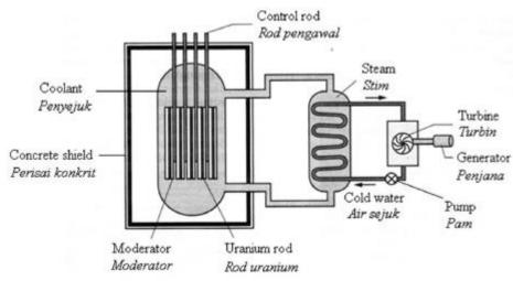
Diagram 23 shows a nuclear reactor which is used to generate nuclear energy.
