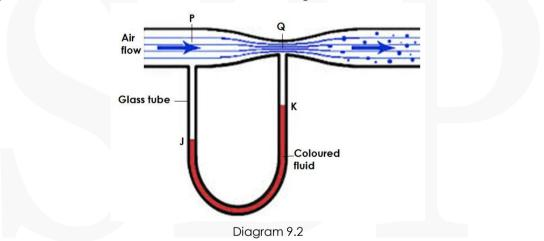
Based on Diagram 9.2, compare the cross-sectional area of venturi tube at P and Q, the speed of air flow at P and Q, and the water level in glass tube J and K.
