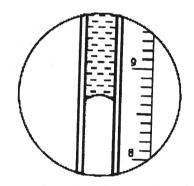
Diagram 1.9 Air column length reading at 60 °C
