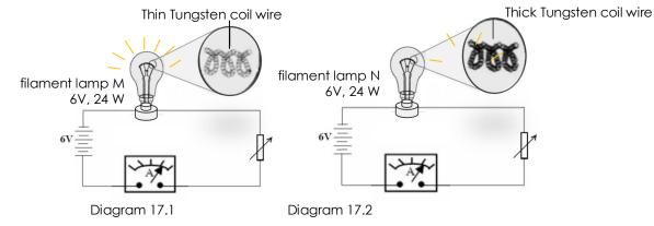
Based on Diagram 17.1 and Diagram 17.2, compare the reading of the ammeter, the brightness of the filament lamp M and N, and the thickness of coiled wire of the filament lamps. Relate the brightness of the filament lamp with the thickness of coiled wire to make a deduction on the relationship between thickness of coil wire and the heat produced by the filament lamp [5 marks]
