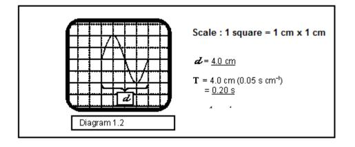
Diagram 1.2 shows the example of illustration of the wave pattern from the CRO screen.
