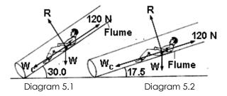
Diagram 5.1 shows the boy sliding down the flume, which is inclined at 30.0° to the horizontal. Diagram 5.2 shows the boy stationary in the flume when the flume is inclined at 17.5° to the horizontal. The frictional force acting on the boy in both flumes is 120 N. Using the concept of force, explain why the boy slides down the flume when the angle of inclination is 30.0° and remains stationary when the angle of inclination is 17.5°.
