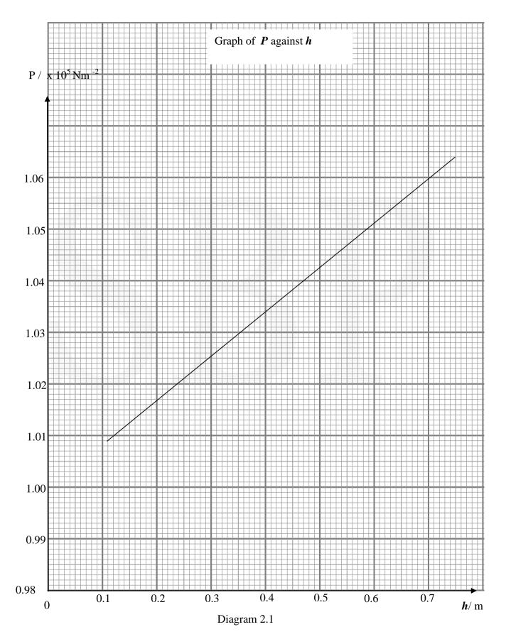
The pressure **P** is determined by using the formula :  $P = P_{\text{liquid}} + P_{\text{atm}}$  where
