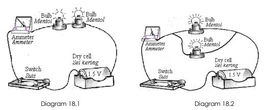
Using Diagram 18.1 and Diagram 18.2, compare the brightness of the bulbs light up, the effective resistance of the type of circuit connections and the reading of ammeter of the both electric circuits.
