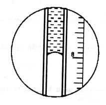
Diagram 1.7 Air column length reading at 40 °C
