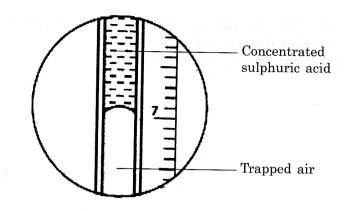
Diagram 1.4 Air column length reading at 0 °C
