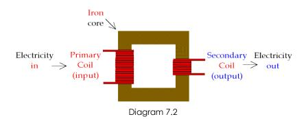
Modification has to be done on the transformer so that it can be used as an efficient 6 V d.c handphone charger.
