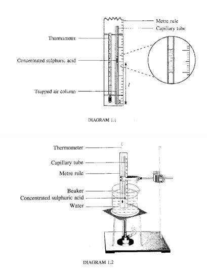
Ice cubes are put into the beaker until the temperature ,  $\theta$  , reaches 0° C. The actual reading of the length of the air column ,  $\ell$ , is shown in Diagram 1.4.
