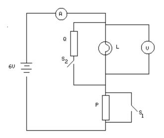
(a) When the switches  $S_1$  and  $S_2$  is opened , the reading of ammeter and voltmeter are 0.3 A and 2.4 V respectively.
