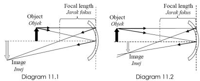
Using Diagram 11.1 and Diagram 11.2, compare the object distance, the size of image formed and the image distance.
