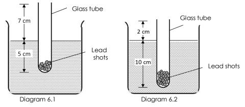
Based on Diagram 6.1 and Diagram 6.2, compare the volume of water displaced by the glass tube, the weight of the glass tube filled with lead shots and the buoyant force acted on the glass tube filled with lead shots.
