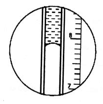
Diagram 1.6 Air column length reading at 30 °C
