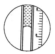
Diagram 1.8 Air column length reading at 50 °C
